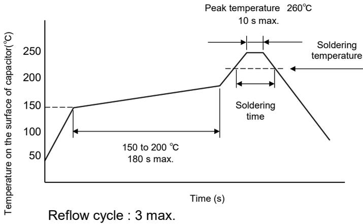
Soldering temperature and soldering time
