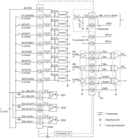
The following pins can be switched by parameters. Input: 5,7,8,9,10,11,12,13 OutPut: 1,2,3,4,25,26
