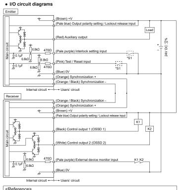
K1, K2: External device (forcible guide relay or magnetic contactor)
