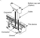
2. Tighten the two M2.6 screws. Tighten to a torque of 0.3N·m or less.
