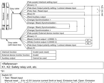
Auto reset ...0 to +2.5V (source current 5mA or less): Émission, Open: Emission halt Interlock setting input, External device monitor input
