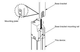
2. With the base bracket in firm contact with the device, tighten the two ultra low-head hex socket bolts [M5 (length 5mm), opposing faces 3mm] that fasten the base bracket. Tighten to a torque of 3N·m or less.
