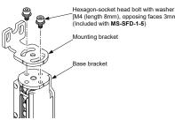
**3.** Install the beam adjustment mounting bracket on the mounting surface with a hexagon-socket head bolt (purchase separately).
