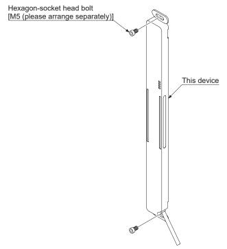
Note: The case of the product is made of resin so the longitudinal dimension is subject to expansion and contraction. When drilling mounting holes, check the drilling locations by positioning the actual product at the installation location.
