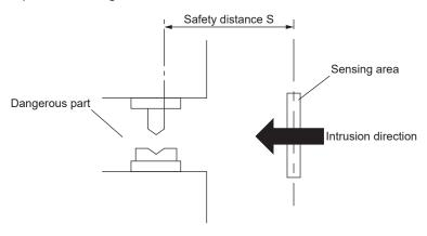
[For use in Europe (EU) (as EN 999)] (Also applicable to ISO 13855) (For intrusion direction perpendicular to the sensing area) <In case that the minimum sensing object is ø40mm or less>
