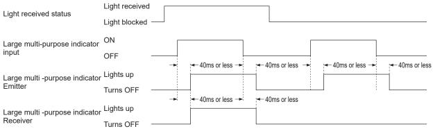
Note: When light from the emitter enters the receiver, the receiver's large multi-purpose indicators will turn ON.
