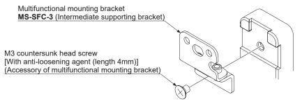
Step 3 Set the multifunctional mounting bracket on the mounting surface using either two hexagon head bolts [M6 (purchase separately)] or four hexagon head bolts [M4 (purchase separately)].
