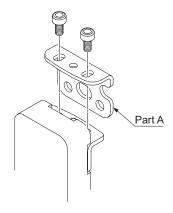
Step 5 Set the multifunctional mounting bracket on the mounting surface using either two hexagon head bolts [M6 (purchase separately)] or four hexagon head bolts [M4 (purchase separately)].
