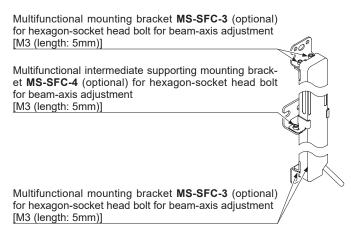
Step 5 Rotate the emitter and the receiver to adjust their positions.
