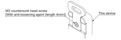
Step 2 Tighten with the M3 countersunk head screw [with anti-loosening agent (length 4mm)]. The tightening torque should be 0.3 N•m or less.
