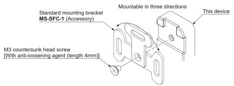
• Set the standard mounting bracket that is ready for setting to the mounting surface using two hexagon-socket head bolts [M5 (please arrange separately)].
