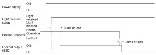
Note: If light from the emitter enters the receiver while the emitter is locked out, lockout information will be communicated to the receiver, causing lockout output (SSD) to turn OFF.
