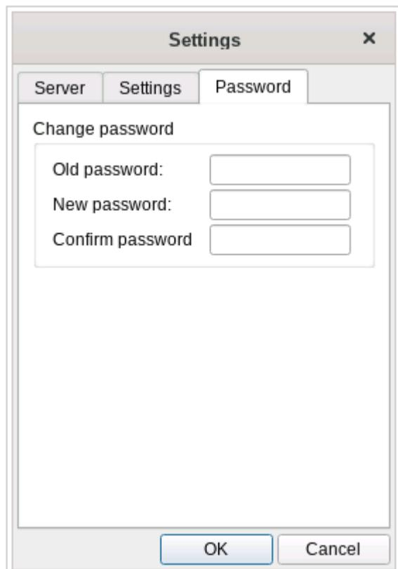
This dialog give the possibility to change the internal password of the HMI device for the admin user (the default password is "admin").
