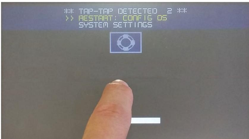
HMI will restart into System Settings in Config OS mode:
