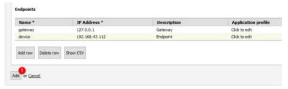
If we are planning to connect also additional devices (e.g. HMI, PLC, etc.), we can repeat previous operations to add the additional Endpoints.
