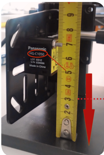
Example: HG-C1050-P Adjusted height 50mm
