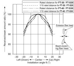
Received-beam amount ratio in Installation (FD-30 / FD-40 / FD-S30 / FD-60)
