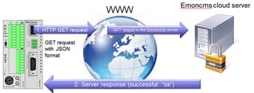
After the server's response the FP WebServer (HTTP Client) writes the content of the reply to the PLC
