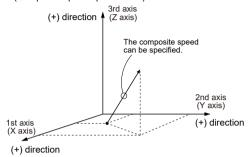
3-axis spiral interpolation (Center point specification/ CW direction/Z-axis movement)
