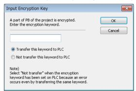
Enter the encryption key and press the [OK] button.Project information is transferred together with the encryption key.
