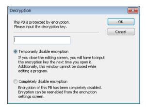
Select a method of disabling encryption, enter the encryption key and press the [OK] button.
