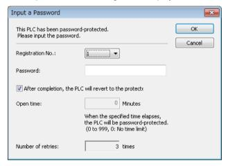
2. Enter the registration number and the password, and press the [OK] button. When the password matches, the project is uploaded from the PLC.
