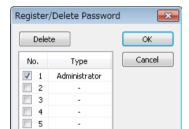
3. Select the No. of the password to be deleted, and press the [OK] button. When the password is that with the registration No. 1, the confirmation message box appears.
