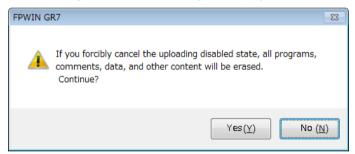
After confirming the message, press the [Yes] button.A message indicating that the settings have been reverted to the factory defaults is displayed.
