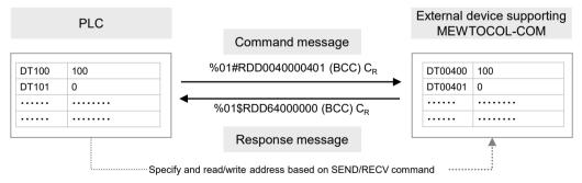
Note: The above figure indicates the data part of MEWTOCOL-COM. In communication via LAN, a header including size information of the sent data is added.
