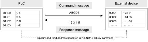
Note: The above figure indicates the data part. In communication via LAN, a header including size information of the sent data is added.
