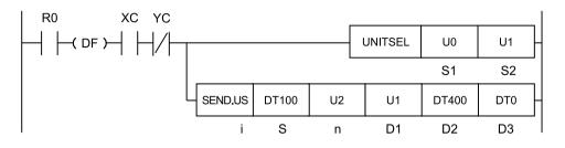
(Note 1) The above figure shows the case that S1=U0 (CPU unit with built-in SCU) and S2=U1 (port number 1) are specified by the UNITSEL instruction.
