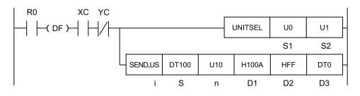
(Note 1) The above figure shows the case that S1=U0 (CPU unit with built-in SCU) and S2=U1 (port number 1) are specified by the UNITSEL instruction.
