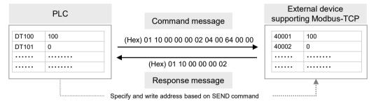
Note: The above figure indicates the data part of Modbus function. In communication via LAN, a header including size information of the sent data is added.
