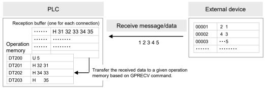
Note: The above figure indicates the data part. In communication via LAN, a header including size information of the sent data is added.
