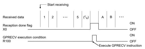
• When the GPRECV instruction is executed, data are copied to the specified area, and the received flags (X0, X1, X2, X3) are turned OFF. The received flags (X0, X1, X2, X3) are turned OFF when I/O refresh is executed at the start of the following scans.
