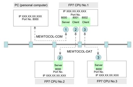
(Note 1) Circled numbers in the figure above indicate examples of allocation of connection numbers.
