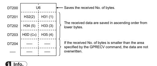
• When a start code and an end code are included in accordance with the communication format of an external device, they are saved as a part of received data in the operation memory. As necessary, insert a program for extracting the relevant data.
