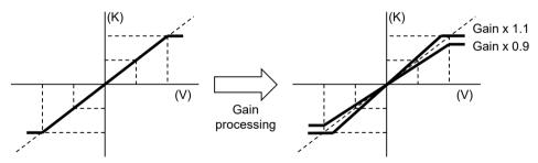
• Offset / Gain processing is executed on a channel-by-channel basis.
