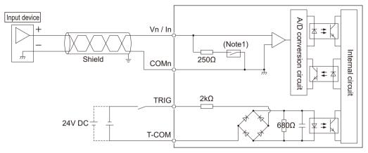
(Note 1) The connection of the circuit varies according to the configuration setting.
