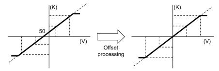
• Gain value settings are used as a function to adjust delicate scale errors between load devices. The gain value slope can be changed in a range of x0.9 to x1.1.
