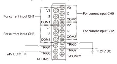
(Note 1) TRIG0 to TRIG3 of AFP7AD4H indicate input terminal numbers. Note that they do not correspond to the analog inputs "CH0 to CH3".
