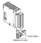
Install the terminal block by inserting it all the way to its original position and pressing the lock button on the bottom of the unit. Then confirm that the terminal block is securely attached and cannot be removed.
