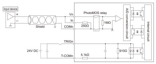
(Note 1) For the current input, connect the V and I terminals.
