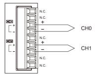
(Note 1) The N.C. terminals are used by the system. Do not connect anything.
