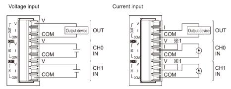
(Note 1) Connect the V and I terminals for using it as current input.
