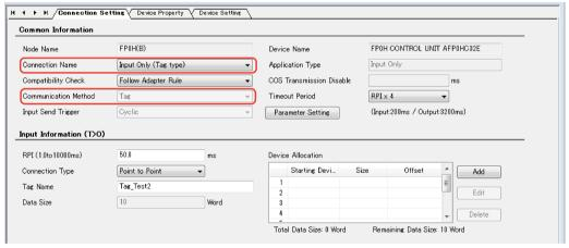
Once "Connection Name" is selected, "Communication Method" (Tag/Instance) will change. In this example, "Connection Name = Input Only (Tag type)".
