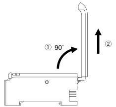
3 Mount the hand-turned knob attached cover **FX-AJ1** from the direction given in the diagram below.
