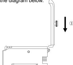
4 Shut the hand-turned knob attached cover. When doing this, make sure to match the cross-shaped projection at the tip of the hand-turned knob into the cross-shaped cavity on the sensitivity adjuster of **FX-311** series.
