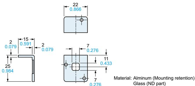
**Mounting drawing with a sensor head**
