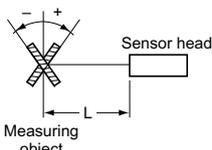
Aluminum vapor deposition surface reflection mirror (0°, ±0.2°)
