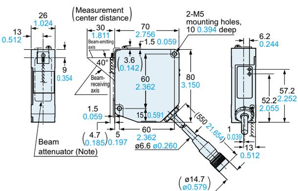
**Setup mode: Specular reflection type**
