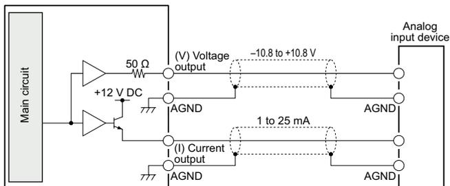
Controller internal circuit ← External connection example
