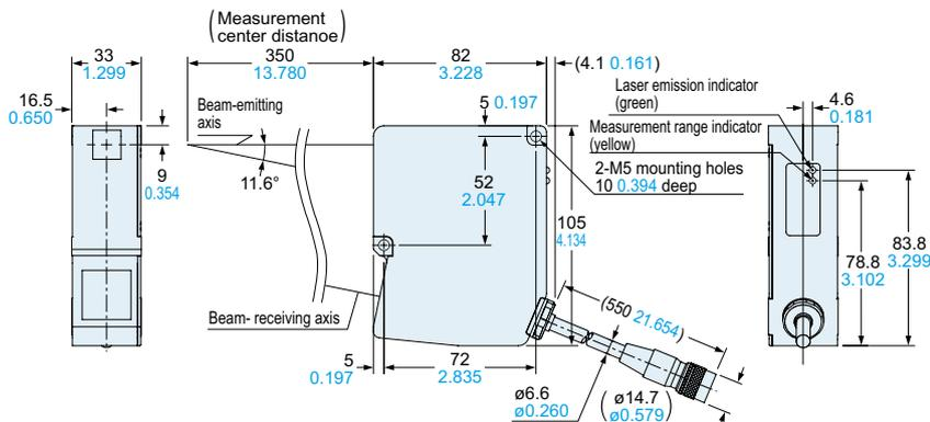
**Setup mode: Specular reflection type**
