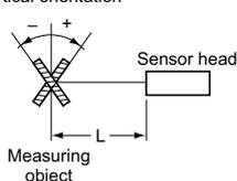
Aluminum vapor deposition surface reflection mirror (0°, ±0.05°)
