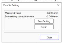
Clicking the [Zero Setting] button in the "Zero Set Setting" dialog box sets a zero setting correction value that assumes the current measured value as zero. Clicking the [Clear] button clears the set zero setting correction value.
