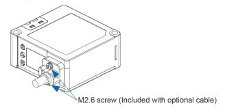
3. When removing the connecting cable from the sensor, loosen the two M2.6 screws, hold the connector part of the cable, and pull out the cable.
