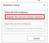
3. If the amount of beam emission is successfully registered using the first workpiece, the amount of beam emission can be registered using the second workpiece. Mount the second workpiece and then click the [Register the amount of beam emission] button. "Registering" will be displayed.
