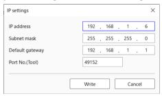
If you have changed the IP settings, click [Write] to write the settings to the sensor, Note that setting duplicate IP addresses for the PC and sensors may prevent the automatic configuration from configuring the IP settings as intended. If changing the IP settings fails, refer to "6.1.1 Configuring sensor IP settings".
