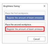
4. If the amount of beam emission is successfully registered using the second workpiece, brightness tuning will be completed. If "Brightness Tuning" is OFF, it will be switched to ON. To perform brightness tuning again, click the [Brightness tuning] button and then perform Step 2 onward.
