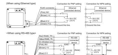
Note: When connecting to the host device, make sure that no potential difference is created between the 0 V side of the power supply for the HL-G2 and the GND of the power supply for the host device. Not doing so may result in accidents or failures in connected devices or this
