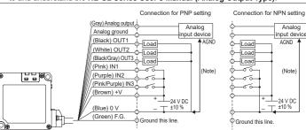
Note: The sensor unit power supply (0 V) and the AGND terminal of the analog output unit are connected within the HL-G2. Make sure that no potential difference is created between the product and external devices. Not doing so may result in accidents or failures in connected devices or
