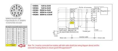
✓ Use the shielded, twisted lines for the encoder cable.
