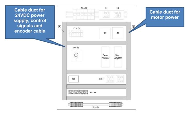
✓ Keeping in mind the recommended distances between individual components according to the manual, make certain the electrical cabinet is appropriately dimensioned.
