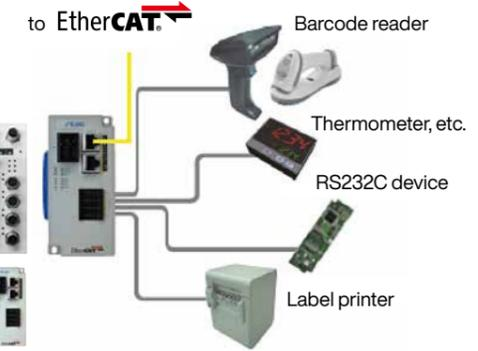
\* IO-Link, Modbus, Serially controlled devices such as RS-232C and RS-485 devices are converted to EtherCAT. EtherCAT can be installed without putting old assets to waste.
