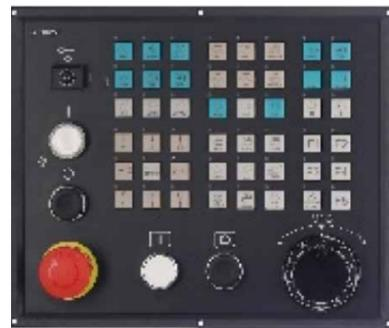
Control Panel for Lathe
