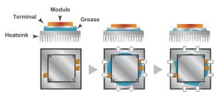
There is no pump-out (dripping, etc.) little change in characteristics
