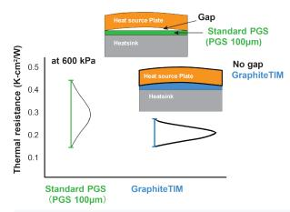
High compression of GraphiteTIM enable to eliminate the gap to reduce the thermal resistance
