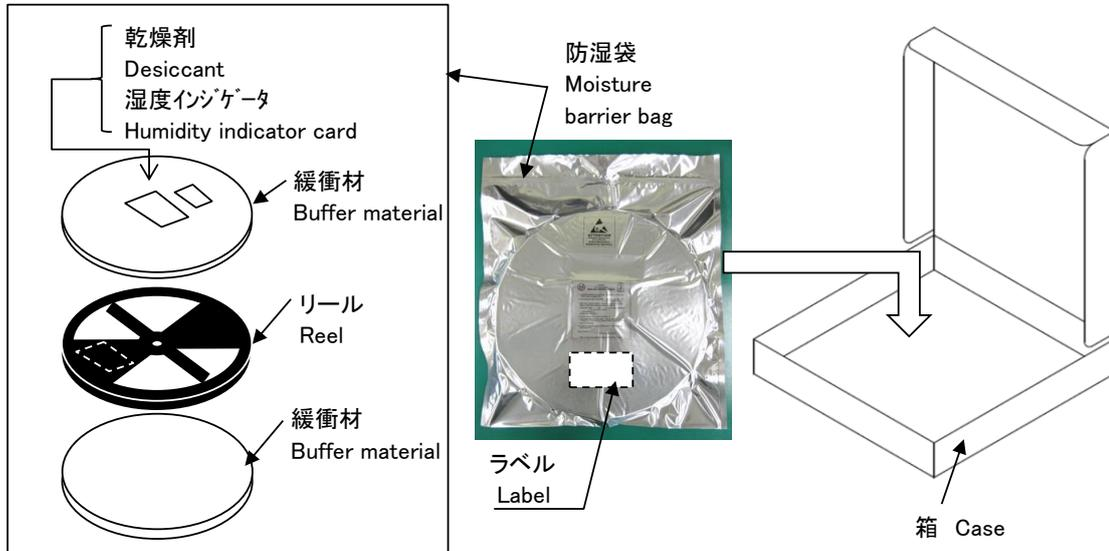
図4-1 内装梱包形態 Figure 4-1 Inside Packing form
