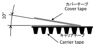
図3 剥離強度測定 Figure 3 Tape exfoliation intensity measurement
