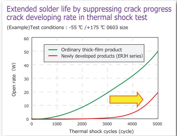
**Guarantees that the resistor endures 1000 cycles of thermal shock testing (-55°C/+175°C)**
