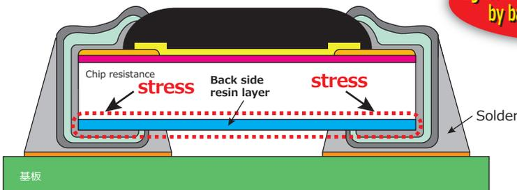
Lighten the stress at solder fillet by back side resin layer
