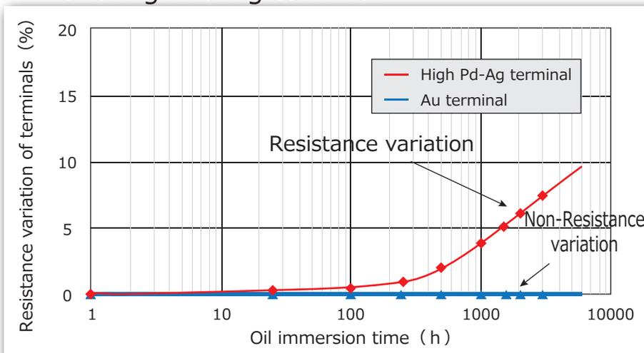
Covered with nickel plating layers, there is no anti-sulfurated characteristic difference between Au terminal and Pd-Ag terminal.
