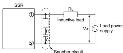
If there is no resistance R (the resistance R controls the discharge current from condenser C), at turn-on of the SSR, there will be a sharp rise in dv/dt and the high peak value discharge current will begin to flow.
