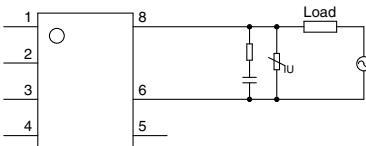
Note: Connection of an external resistor, etc., to terminal No. 5 (gate) is not necessary.
