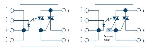
SSRs in particular are an ideal choice for application where AC loads have to be switched repeatedly without creating noise, such as temperature control. This is due to the nature of the triac on the output side: A triac is a four-layer diode with three terminals which can conduct current from anode to cathode and vice versa. It is non-conductible until a current pulse of about 50 mA is applied to its gate. The triac then conducts the load current till the current drops below a certain level.
