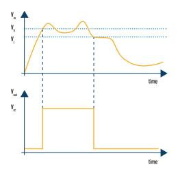
voltage drop across RE. This makes it easier for transistor T1 to reach the saturation region and turn into on-state. Consequently, the output voltage Vout also rises. If the input voltage drops below the lower threshold value VI, the transistor T1 turns off and T2 turns on, forcing the output voltage Vout to drop.
