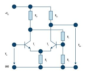
of a resistor and a thermistor acting as the input signal. If there is no input voltage, the transistor T1 is in the off-state. The voltage divider R1 and R2 instead directs current to the base of transistor T2, causing current to flows through T2 and RE. If the input voltage Vin exceeds the threshold value, current flows through T1 and the voltage drop across the voltage divider R1 and R2 gets lower, reducing the base current of T2 and
