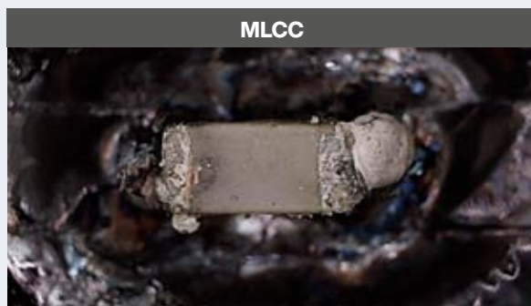
PCB burned due to continuous short-current
